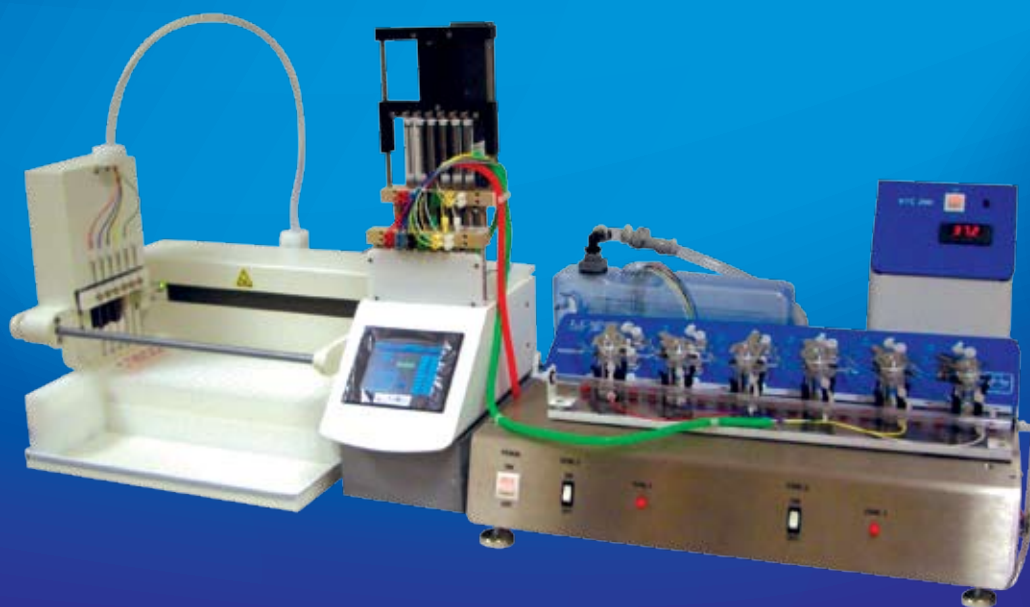
Automated Transdermal Syringe Pump Sampling System
