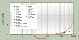
Total power error with rated range input for an arbitrary power factor (at 50/60 Hz)
