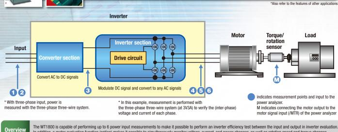
In addition, a motor evaluation function (option) makes it possible to simultaneously monitor voltage, current, and power changes, as well as rotation speed and torque changes.
